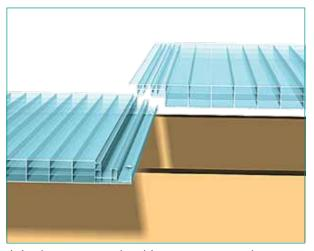
Join the next panel, taking care to match the male / female profiles before applying pressure. Ensure that panel is fixed.
